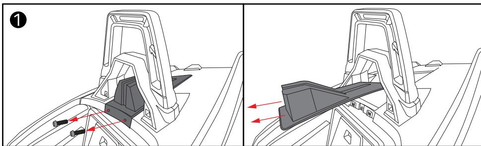
**Remove the factory rear hoop accent using a T40 TORX socket to extract the (2) screws on bottom of the piece and a T25 TORX to extract the (2) screws on top of the piece and pull it to the font, then using the T40 TORX to extract the (2) screws in the back of the piece and pull it to the back. (Picture 2)**
