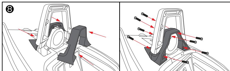
This kit needs an aftermarket amp pre-installed with the speaker wires in this location, only after this step can you install the speakers using the aftermarket amp's speaker wire and RGB LED wires (optional) of the LED module (LED -BTC not included). Secure the speakers using stainless steel screws and tighten them, be careful not to over-tighten or the hole may be damaged and not properly secure the speakers.
