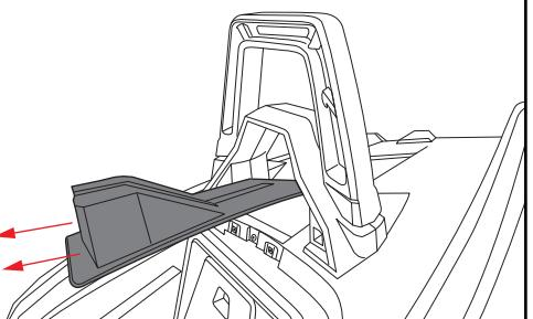
Proceed by removing the factory rear hoop accent. Start by using a T40 TORX socket to extract the (2) screws located at the bottom of the piece. Then, utilize a T25 TORX socket to remove the (2) screws positioned at the top of the piece. Gently pull the accent towards the front. Then, use the T40 TORX socket to extract the (2) screws located at the back of the piece, and pull it towards the back to fully detach it. **(Picture 2)**
