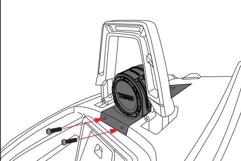
Re-install the rear hoop accent following the reverse procedure of the removal. Ensure the accent is positioned correctly, then secure it by reattaching the screws in the same locations as before.(Picture 4)
