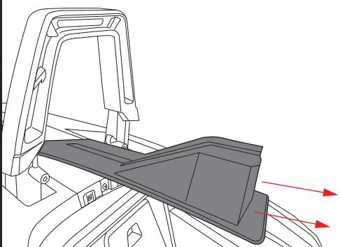
Now, carefully slide the new speaker pod in place and secure it using the factory T25 bolts on front bottom of the piece, then re-install the Ring-Nut and the gas cap. (Picture 7)
