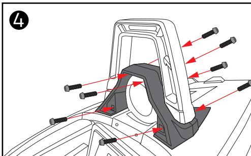
Begin by removing the factory rear hoop accent. Use a T40 TORX socket to extract the (2) screws located at the bottom of the piece. Then, utilize a T25 TORX socket to remove the (2) screws positioned at the top of the piece. Pull the accent towards the front. Then, use the T40 TORX socket to extract the (2) screws located at the back of the piece, and pull it towards the back to fully detach it. (Picture 5)
