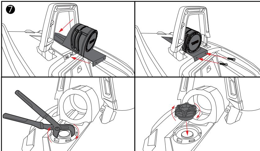
Re-install the rear hoop accent following the reverse process of removal. Ensure that the accent is aligned correctly, then use the appropriate screws and sockets to secure it back into place. (Picture 8)
