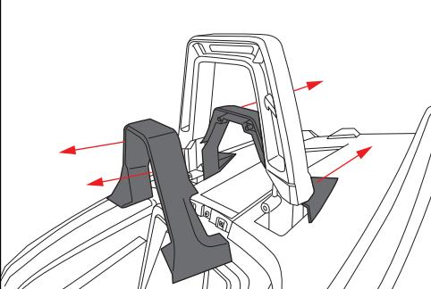
Install the new speaker pod following the same procedure used to remove the factory component. Position the pod in place and secure it using the factory T25 bolts located on the front bottom of the piece. **(Picture 3)**
