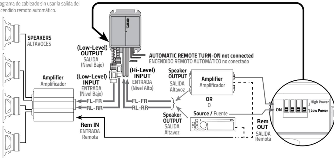
**DOUBLE STEP-DOWN RATIO** High-Power (6.5:1) and Low-Power (4:1) step down conversion ratio selectable via DIP switch independently for each input, front and rear, for a correct interface with both OEM or aftermarket sources up to 50 Watts (Low Power) 100 Watts (High Power).
