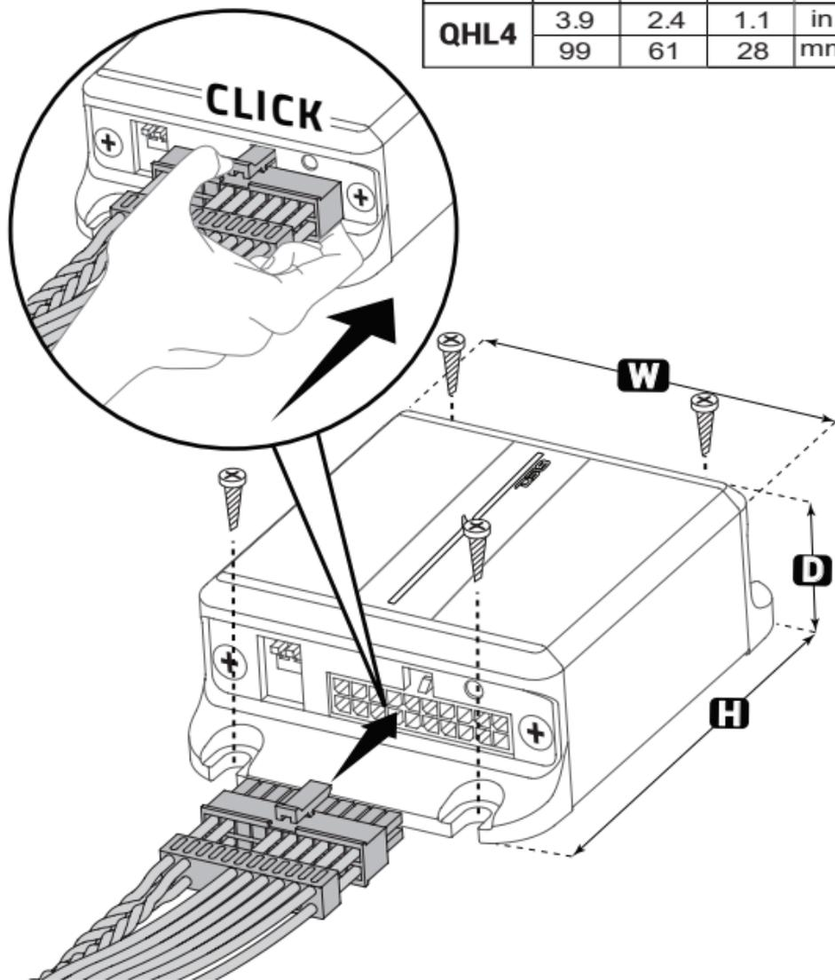
**UNIVERSAL SPEAKERS SIMULATOR** It simulates the load of the speakers on the input 2 channels (Front or Rear), for a complete compatibility of the interface with OEM sources that detect the original speaker load (impedance) connected to their outputs.
