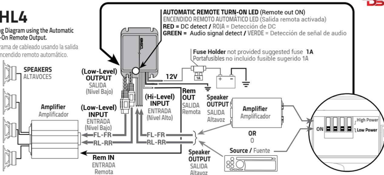
**DOUBLE STEP-DOWN RATIO** High-Power (6.5:1) and Low-Power (4:1) step down conversion ratio selectable via DIP switch independently for each input, front and rear, for a correct interface with both OEM or aftermarket sources up to 50 Watts (Low Power) 100 Watts (High Power).
