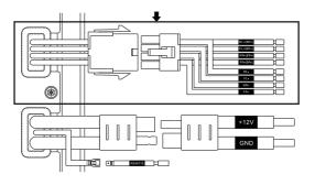
while being careful that there is no loose or frayed strands of wire and tighten the Allen head screw down on the terminal till the wire is tightly secured in place. If the wires ever come in contact with each other the amplifier will go into protection.
